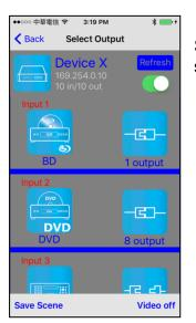
Slide left from load scene page to enter output selection mode (support multiple selection)
