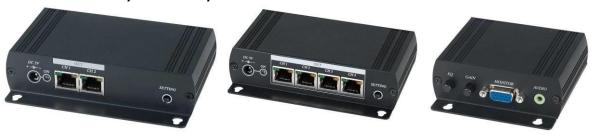
VE02AL, VE05AL is designed for VGA +Stereo Audio signal over cost effective CAT5 cable to instead of VGA and Audio cable. VE02AL receiver built in chainable output to cascade the other receiver for working range over 300 meters. It is optimum video performance under long cable run and perfect for multiple monitor display.
