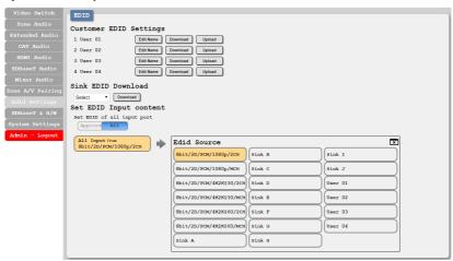
Appoint/All: The Set EDID Input Content section allows for the assignment of an EDID to each individual input port, or to all inputs at once. Click the selection bar to toggle between "Appoint" (individual assignment), or "All" inputs.
