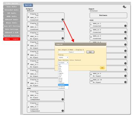
■ **Test Pattern Color Control:** The test pattern type can be changed to any one of sixteen different options. The patterns include full screen colors as well as a selection of other basic patterns.
