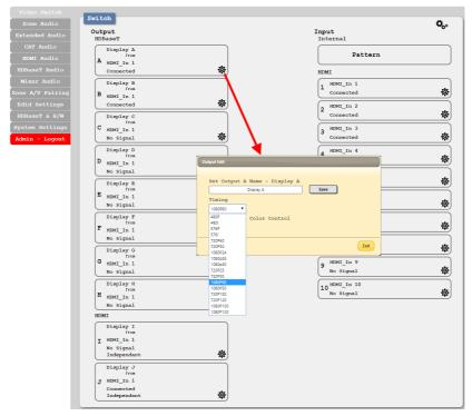
■ **Timing:** Test patterns can be generated on either the HDMI or HDBaseT outputs at the following standard resolutions with a variety of refresh rates: 480i/p, 576i/p, 720p, 1080p, 4K. Test
