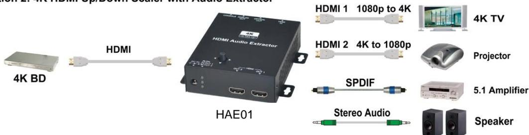
**HDCP 2.2 to 1.4 and 4:4:4 to 4:2:0 and Up/Down Scale Capable
