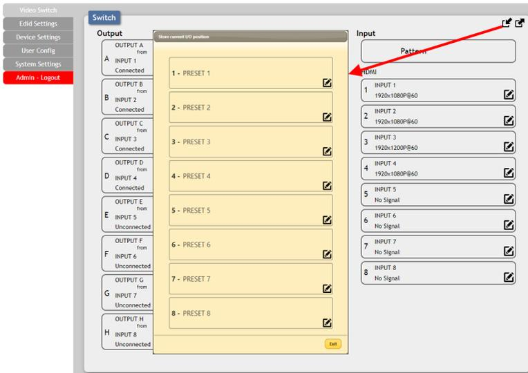
**5) Preset Settings:** This matrix can store up to eight video routing presets. Presets can be utilized to store multiple different routing states in advance for rapid, hassle-free, recall.
