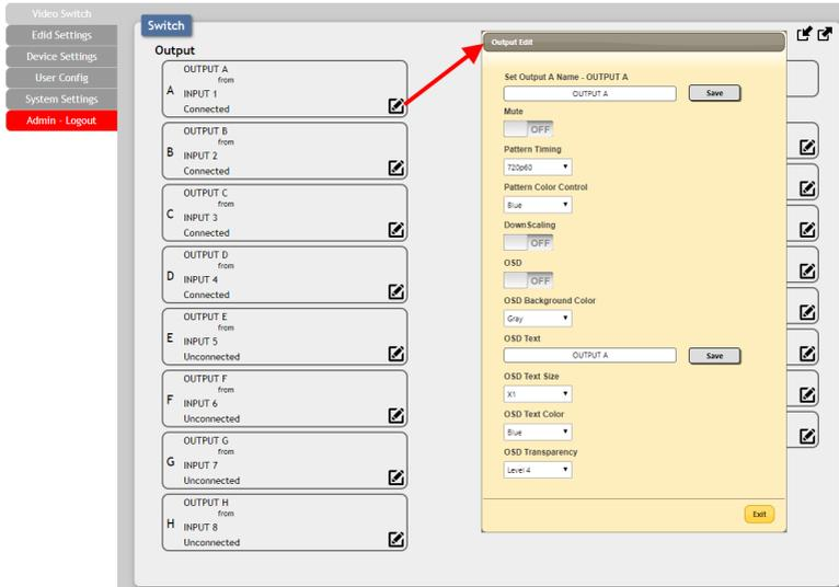
3) **Output Edit:** A variety of output settings, including name, muting, test pattern configuration, downscaling, and OSD options can be configured here. Please click the “Edit” icon (✎) within the Output button to open up the Output Edit window.
