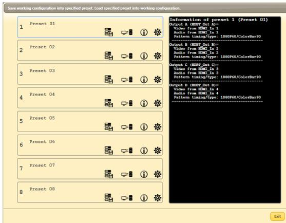
**4) Preset Settings:** This matrix can store up to eight routing presets. Presets can be utilized to store multiple different routing states in advance for rapid, hassle-free, recall. To store, recall or view a preset, click the "Preset" icon (
