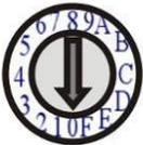
HKM01-4K built in rotary switch for pairing devices and the rotary switch can be used to switch 0-F channel pairing with group setting of switch 1. The channel number and group setting of the transmitter and receiver must be same to be connected each other, total up to 32 (16 for each group) pairs could be setup at one switch.
